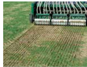
TriWave technology creates the optimum slits for improved seed-to-soil contact, while minimizing turf disruption.
