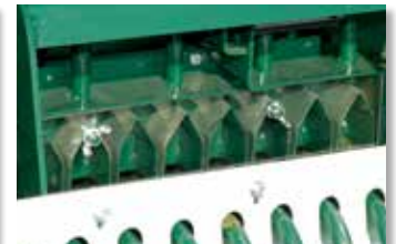
Patent-pending seed diverter increases germination by placing seed directly into the slit.
