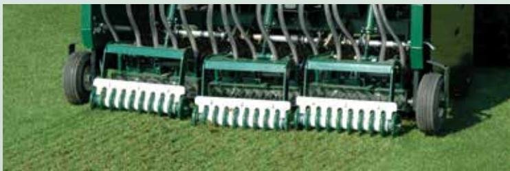
Floating heads follow the ground contour.
