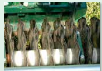
WaveBlade technology creates optimum slits, increasing seed-to-soil contact.
