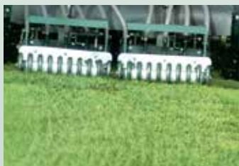
Patented floating heads follow the contour of the ground, optimizing seed-to-soil contact for better germination.
