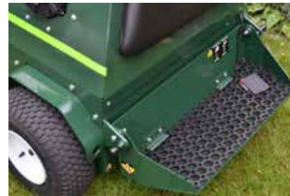
Cushioned platform reduces vibration without sacrificing traction. Also locks up for easy access to the tines.
