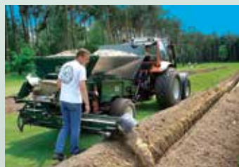
The swivel kit locks in any position or can be moved 180° by hand.
