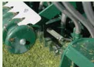
Depth adjuster allows you to adjust to varying conditions or seed types.
