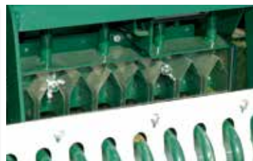
Patent-pending seed diverter increases germination by placing seed directly into the slit.
