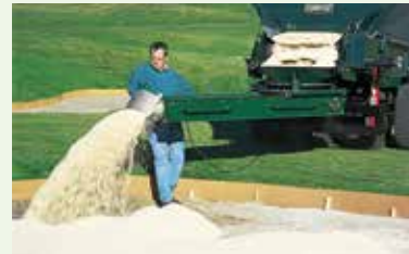
Cross conveyor with 180° swivel action allows you to place material right where you want it.
