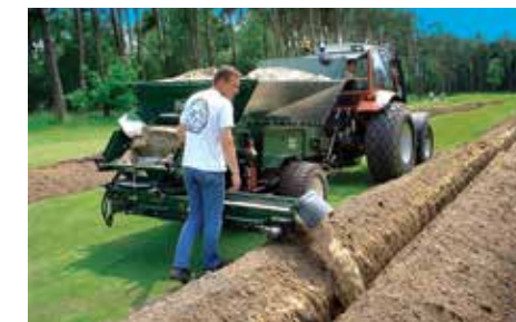
The swivel kit locks in any position or can be moved 180° by hand.
