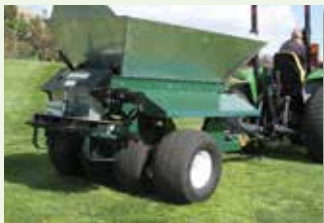
Four-wheel walking beam suspension.
