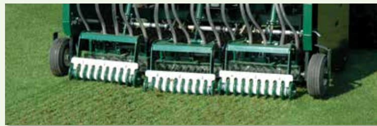
Floating heads follow the ground contour.
